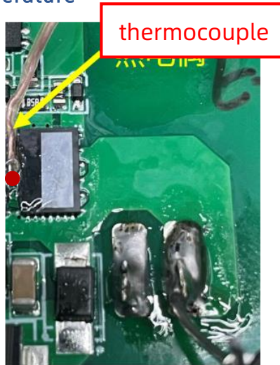
Figure 69 Thermocouple test point
